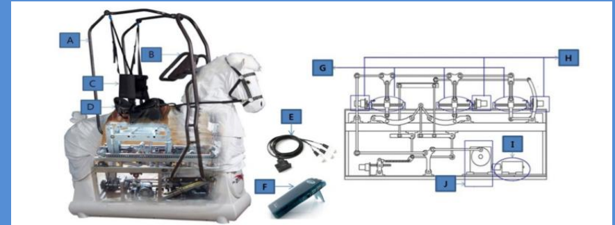
Fig. 1. Robotic hippotherapy system and experimental setup. A: suspension frame, B: controller, C: harness, D: saddle, E: 3-axis accelerometer sensors, F: LabPro interface, G: ball screw, H: servomotor, I: pulley, J: main motor.
